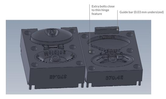
Inlet. Clamping action of the injection molding machine will act to seal the parts further against each other
