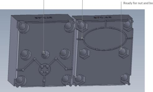
Vacuum relief tracks connecting outlets to the surface beyond the build plane during printing
